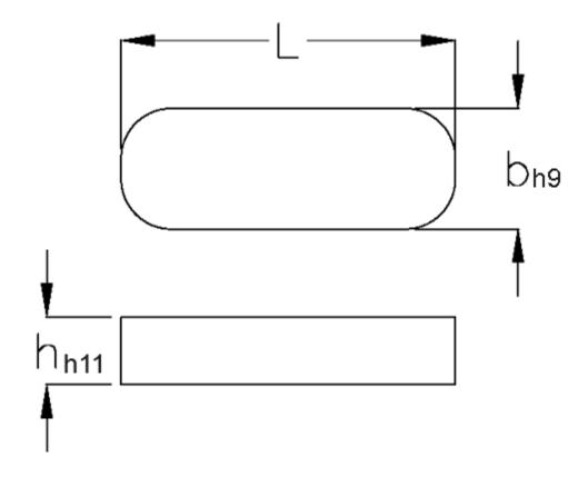
$\begin{array}{ll} b & = 5 \\ h & = 5 \\ L & = 36.0 \\ Tolerance \ b = 0.030 \\ Tolerance \ h = 0.075 \end{array}$
